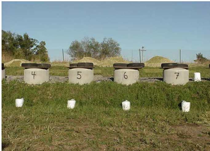
Figure 2. View of midi silos positioned on sloping hill to allow for external collection of effluent.
