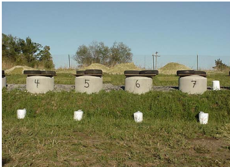
Figure 3. View of midi silos positioned on sloping hill to allow for external collection of effluent.
