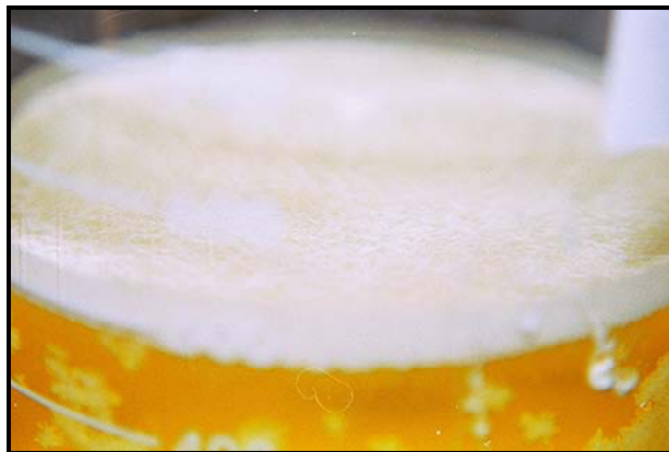
Figure 2. Growth of lactose crystals on the surface of batch 3 (day 5).
